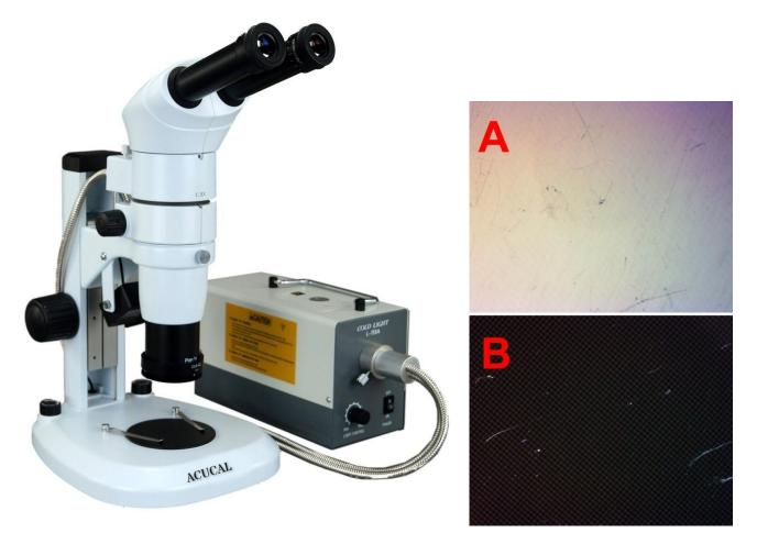
Image A and B are a cellphone screen under our CMO stereo zoom microscope. Image A is by the EPI coaxial illuminator, in which all scratches can be seen clearly with all details and Image B is by the conventional incident light, in which only a few of the scratches can be seen with no details.
